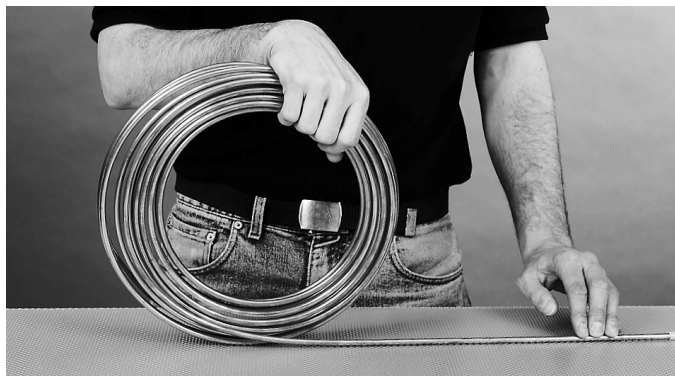
Figure H. Uncoil Tubing without Creating Bends
