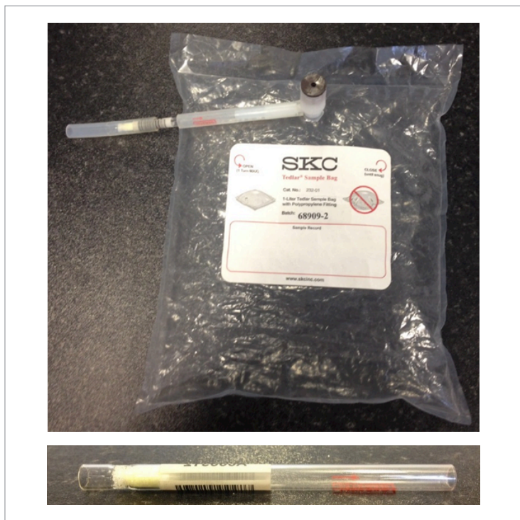
Figure 3: Fritted thermal desorption tube, filled with cage material and attached to filled 1 L Tedlar bag.
