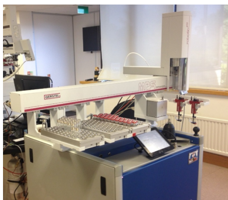
Figure 1: Syft Technologies Voice200 ultra SIFT-MS with GERSTEL MPS Robotic autosampler.
