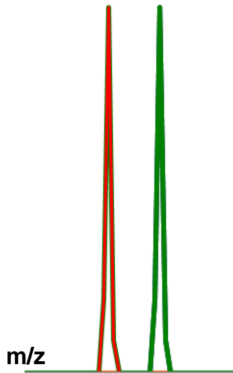
Two mass peaks with FWHM 0.05 u with 0.5 u between centroided m/z value
