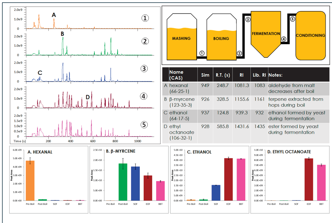
Figure 1. Various points during the brewing process (labeled 1 through 5) were monitored with GC-MS. Representative chromatograms at each processing point are shown. Example analytes that clearly changed during the brewing process are also shown (labeled A through D).
