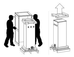
The generator can now be lifted out of the crate base and onto the floor. This should be done again with someone positioned at either side. There is a gap in the foam base for hand access, one hand should be positioned here underneath the generator and the other at the back supporting the weight. The generator should then be tilted back slightly and then up and out of the foam base and onto the floor.
