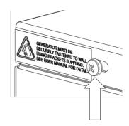
Locate the screw in the top rear corner of the unit, beside the yellow warning label. Remove the screw from the generator this should be repeated for the other side of the unit, and retain.
