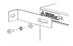
Next, using the screw which was removed, fit the bracket and washers provided to the generator. Again this should be repeated for the other side. The bracket is adjustable to accommodate varying kickboard widths.
