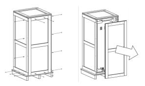
Now, with someone positioned at either side of the shipping crate, the top half of the crate can be slid backwards and away from the rest of the crate. With the top of the crate removed the foam insert of top of the generator should also be taken off.
