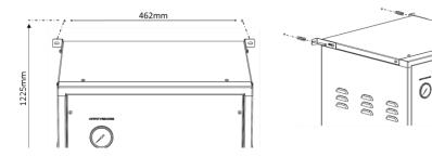
Finally, using the dimensions provided, fix the wall plugs to the wall, ensuring wall plug is suitable for the type of wall. If not, use the correct type. Secure the generator to the wall with the screws from the fittings kit.
