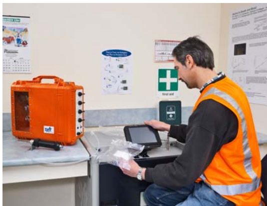
Figure 3. Syft Technologies' Sample Case holds three 1-liter Tedlar or Kynar sample bags, which are removed for Voice200 analysis as shown. The operator uses the integrated touch screen display to start testing and to view results.
