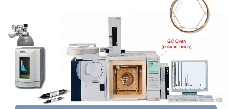
A GC column is the heart of a GC system (where the chromatographic separation occurs).
