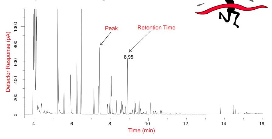
A chromatogram is the result of a GC separation.
