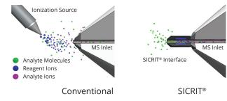
The patented SICRIT® ion source extends the inlet of your MS and ionizes all molecules drawn in by your MS by means of a specially shaped cold plasma. The plasma is ignited within a capillary, thus transmission and, consequently, sensitivity are greatly improved.
