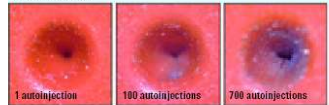
Agilent BTO Septa With CenterGuide: Very Little Coring Even After 700 Autoinjections
