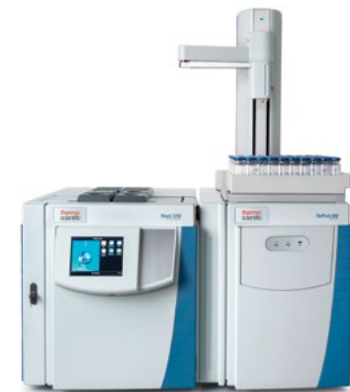
TriPlus 500 Headspace Autosampler coupled to the TRACE 1310 Gas Chromatograph
