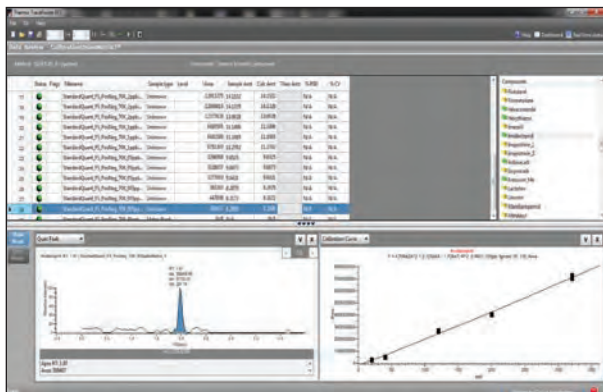
Figure 2. TraceFinder software displays imidacloprid calibration curve plot of matrix, R^2 , list of compounds, and chromatogram. A green flag in the compound list indicates the compound was found in the unknown sample, whereas a yellow flag indicates the compound was not found.
