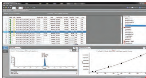
Figure 4. TraceFinder software displays diuron calibration curve plot of matrix, R^2 , list of compounds, and chromatogram. The highlighting of diuron in the upper right section indicates that the compound was found within the calibration curve. Therefore, there are no flags present next to the name.
