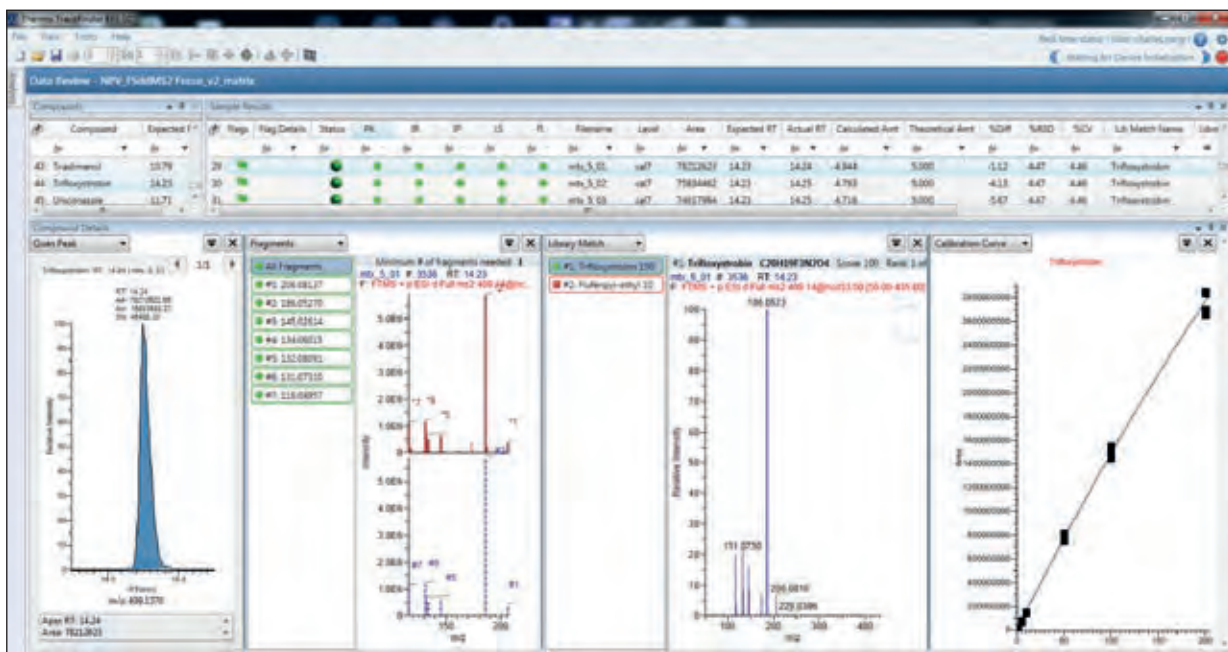
Figure 5. Trifloxystrobin at 5 ppb, showing compound details in lower portion to highlight quick data review.
