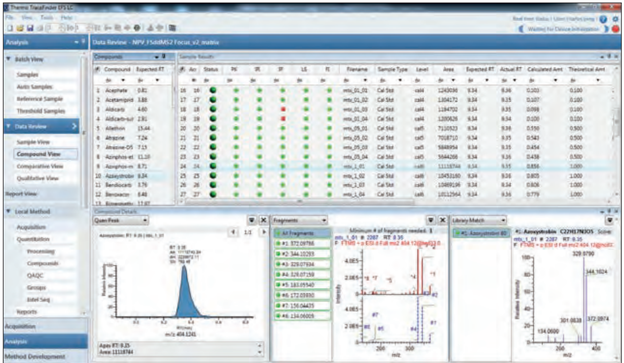
Figure 10. Azoxystrobin library match confirmation with fragmentation confirmation at 1 ppb, showing a library match score of 80% confidence in the lower right pane.
