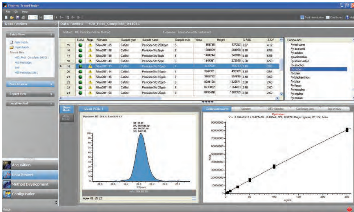
Figure 4. TraceFinder software view of extracted ion chromatogram and solvent standard calibration curve [metalaxyl (A) and pyridaben (B), 10 µg/L, 3 replicates, quadratic curve fit]
