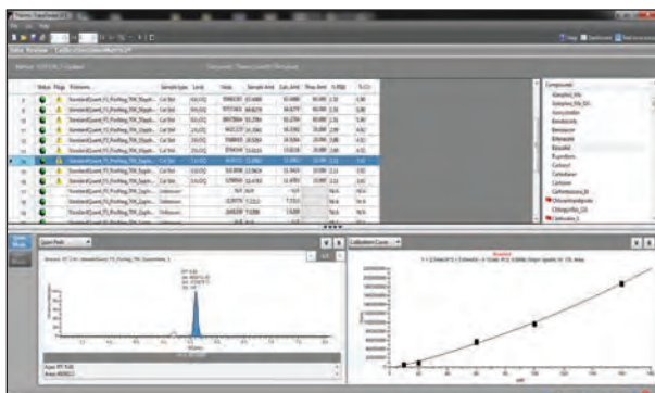
Figure 3. TraceFinder software displays boscalid calibration curve plot of matrix, R^2 , list of compounds, and chromatogram. The red flag indicates the compound has an issue with the calibration curve and that it did not meet the flagging requirement. The yellow triangle caution sign indicates there is an issue with a single or multiple compounds in the sample that needs to be checked.
