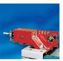
• The **GERSTEL Online TDS G** is designed for continuous monitoring of compounds in air, gas streams or large volume headspace. The TDS G features automatic sample volume control and reversed sample desorption flow.
