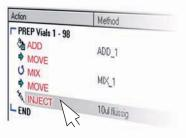
MAESTRO Software enables Sample Prep by Mouse-Click. All sample preparation steps are conveniently and easily selected from a drop down menu and added to the method. Example:
