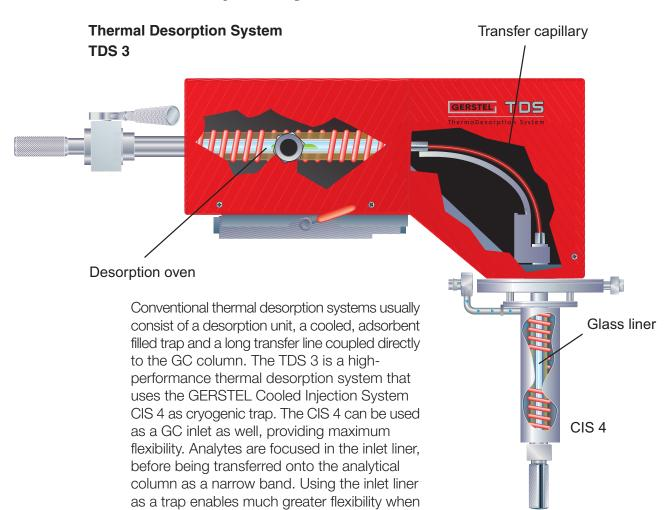
Prior to desorption in the TDS 3, tubes can be cooled and purged with carrier gas to remove oxygen, water or unwanted solvents. Two temperature ramps enable programmed heating and stepwise desorption of analytes up to 400 °C. Analytes are transferred at high flow through a very short transfer line (15 cm long) from the TDS 3 to the CIS trap for best possible recovery.
