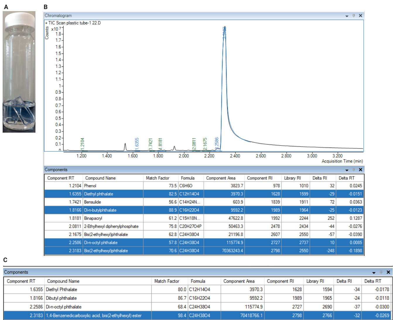
Figure 3. (A) Plastic tube extraction with acetone; (b) Unknowns Analysis results for the plastic tube analyzed against the custom spectral library; (C) selected Unknowns Analysis results for the plastic tube analyzed against the NIST spectral library.
