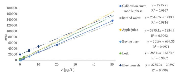
**Figure 5.** Comparison of the slope of the external calibration curve with the slope of the standard addition curve.
