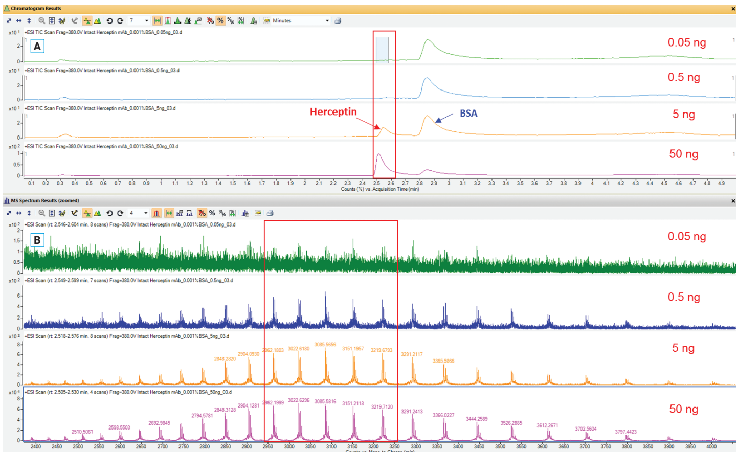
Figure 2. (A) Representative total ion chromatograms (TIC) of various amounts of intact Herceptin analyzed in the neat solution. (B) The corresponding charge state distributions of the targeted mAb.
