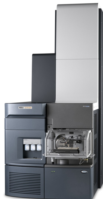
Xevo G2-XS QToF fitted with a 2D DESI stage.
