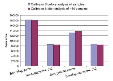
Figure 17. Peak areas for calibration standard 6 remain constant even after analysis of more than 50 samples.
