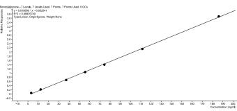
Figure 12. Calibration curve for benzo[a]pyrene, 3.1-186 ng/mL.
