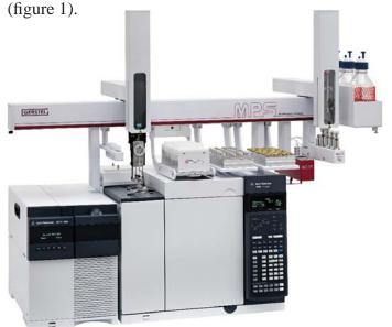
Figure 1. GC/MS system used for automated determination of benzo[a]pyrene and benz[a]anthracene in tar distillation products.
