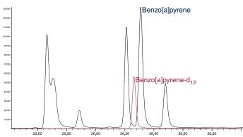
Figure 8. Benzo[a]pyrene in sample C, SIM, m/z 252: 264.
