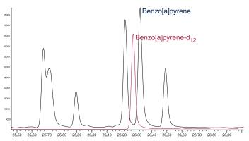
Figure 7. Benzo[a]pyrene in sample B, SIM, m/z 252: 264.
