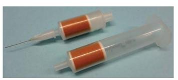
Figure 2. Top: Standard solid phase extraction (SPE) cartridge adapted for automated SPE with the GERSTEL MPS. Such cartridges are commercially available from a number of vendors. Bottom: Standard solid phase extraction cartridge.
