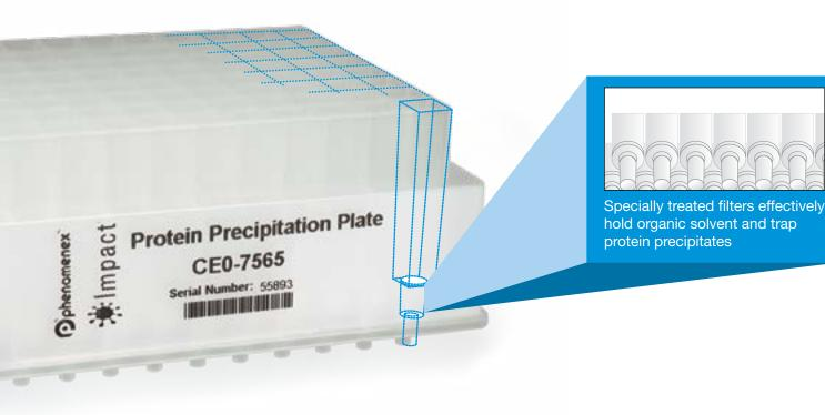
Impact protein precipitation plates with Solvent Shielding Technology™ offer a rapid and convenient way to remove proteins from plasma and tissue samples prior to analysis. The Solvent Shielding Technology design will withold organic solvents above the filter membranes for up to 25 minutes, allowing for direct in-well precipitation upon sample addition. The precipitate is then filtered out via vacuum, centrifuge or positive pressure resulting in a clean, protein depleted extract.
