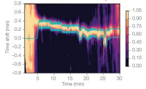
Adaptive RT routine in action: An example of the acquisition cycle outlined using the DIA mapping function to detect, evaluate, and align the retention time windows following the completion of every other cycle. The teal lines show the leading and tailing edges of the tMSn events with automatically determined time shifts. The various colors are associated to the dot product overlap of RT features mapped in real time versus the Alignment Map file.
