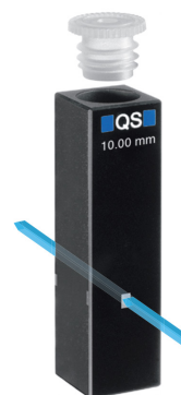
Figure 6. A highly focused beam of 1.5 mm width delivers maximum accuracy.
