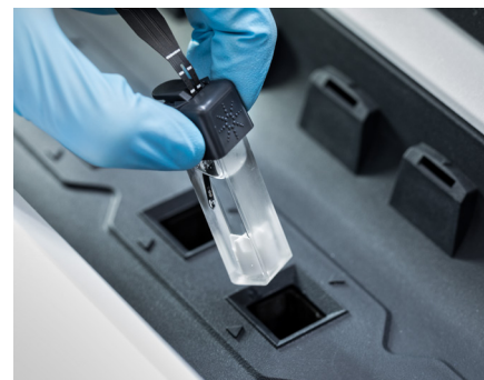
Figure 8. The unique Agilent Cary 3500 UV-Vis in-cuvette temperature probe has a superfast feedback loop. The probe provides instantaneous temperature readings, direct from the sample.
