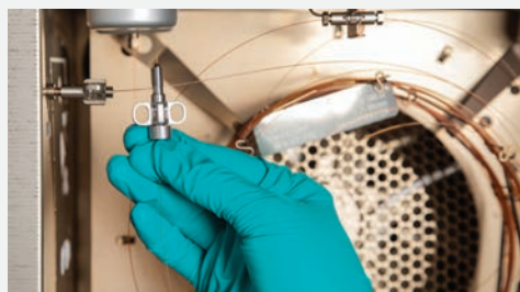
Self-Tightening column nut Installation – Inlet and Detectors video:
