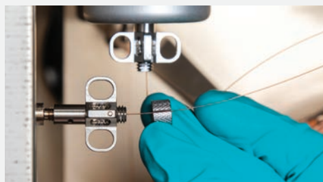
Self-Tightening column nut Installation – MS interface video:
