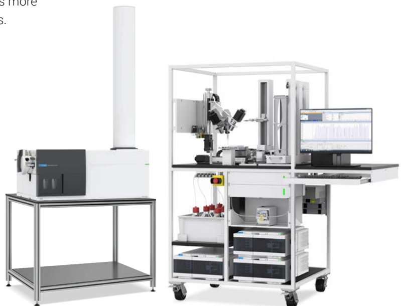
The RapidFire 400 can be connected to TOF, Q-TOF, or triple quadrupole MS.
