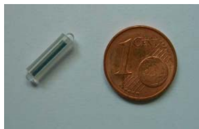
Figure 1. Twister PDMS stir bar, 1 cm length, 1 mm phase thickness.
