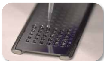
Fig. 1 FlexiFocus slide: influence of the chemically modified surface on the containment of the sample droplet.
