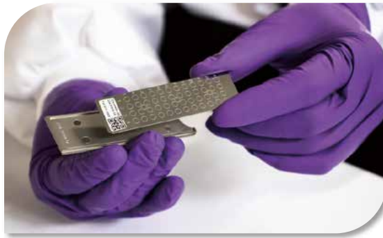
Fig. 5 FlexiFocus adaptor and insert: four circular-shaped magnets snap insert into place.
