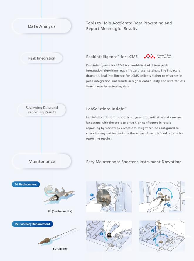
The RX Series keeps the same user-friendly maintenance as its predecessors. Changing the ESI capillary and the desolvation line (DL), which transports ions into the vacuum region, are designed for quick and effortless replacement without breaking vacuum helping to reduce time spent on maintenance and increase instrument uptime.
