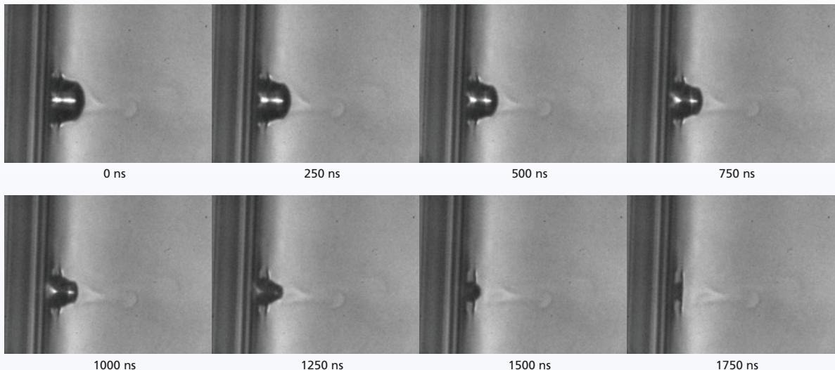
Recording speed: 20 Mfps, Field of view width: approx. 110  $\mu\text{m}$
