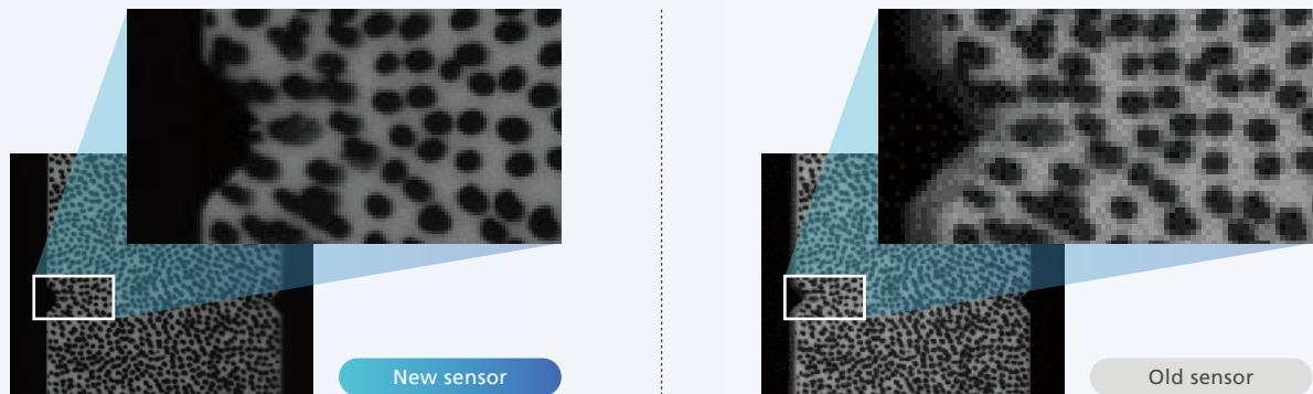
The new image sensor has three times the number of pixels and six times the amount of memory thanks to a reduction in memory size. This technology is used to achieve an improved image resolution of 300,000 pixels with no negative effect on
