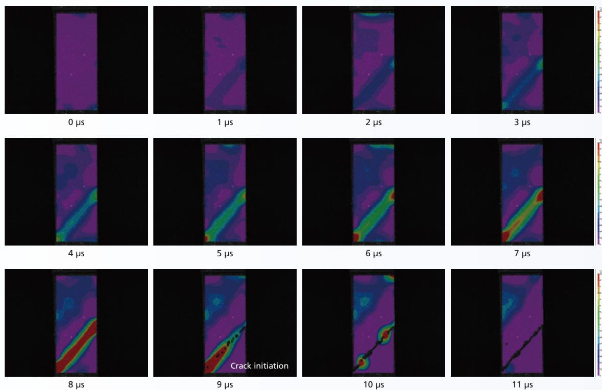
Recording speed: 20 Mfps, Test speed: 10 m/s, Specimen width: 12 mm
