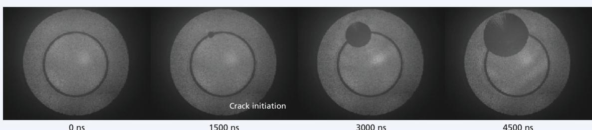
Recording speed: 10 Mfps, Field of view width: approx. 45 mm
