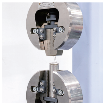
5 kN Non-Shift Wedge-Type Grip File Teeth for Flat Samples T14-21
