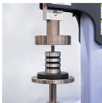
Upper: Fixed Compression Plate 100 mm Dia. Lower: Lower Compression Plate 118 mm Dia.
