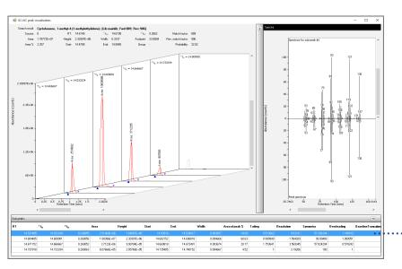
Fast and simple review of peak merging allows sub-peaks to be compared quickly by scrolling through the table, with any issues seen at a glance.
