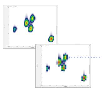
The familiar interpolation can be applied to give colour plots (left), but the raw 'nearest neighbour' view (right) shows the actual slices, e.q. for verifying the optimal number of modulations per peak.
