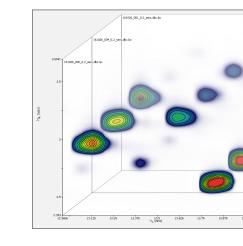
Contour lines and perspective overlays enable differences between multiple chromatograms to be easily visualised.
