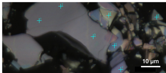
Figure 1. A comparison of bulk and manually exfoliated, 2D MoS 2 shown in common-scale. The in-plane E'₁ 2g peak shows the same intensity in both crystals while the out-of-plane A'₁ g peak decreases by a factor of 2.8 in the 2D crystal.
