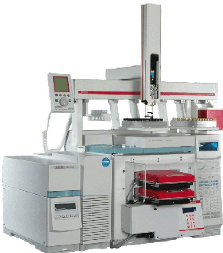
Figure 3. Dual column MACH connected to 6890 GC system.
