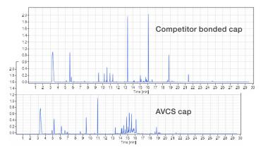
Chromatograms show the background peaks for two different cap technologies (shown in the same scale). Less background peaks result from the AVCS cap compared to the competitor bonded cap.
