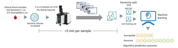
Samples of bacteria were analyzed for strains that display drug resistance following this simple workflow with the Agilent Cary 630 FTIR spectrometer. Bacterial samples were placed directly onto the ATR without the need for drying. The time for sampling and spectrum collection was under 5 minutes per sample, which is significantly shorter than the time needed for genome sequencing using the current gold-standard technology.
