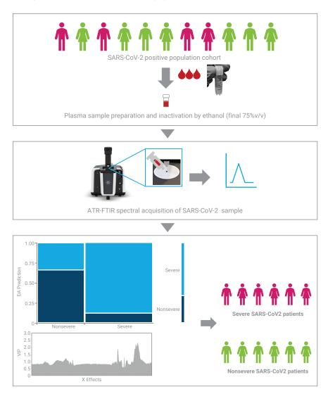
The severity of COVID-19 was assessed through this simple workflow, where plasma samples can be analyzed using ATR-FTIR spectroscopy with the Agilent Cary 630 FTIR spectrometer.
