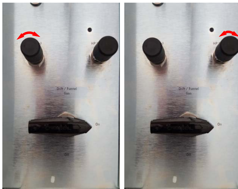
Figure 6. Adjusting the Drift Cell pressure regulator (left) and High Pressure Funnel pressure regulator (right)
