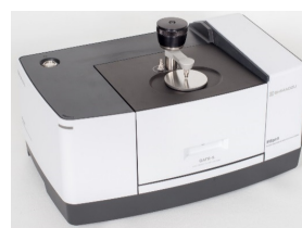
Fig. 4 IRSpirit with QATR-S Single-Reflection ATR Accessory (Diamond prism)
