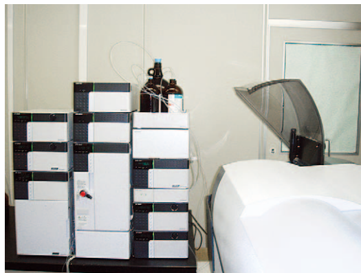
Fig. 2: Photograph of 2D-LC/MS Impurity ID System
