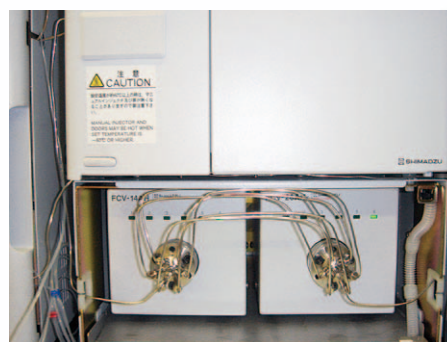
Fig. 5: Fractionation Loop Valve Unit
