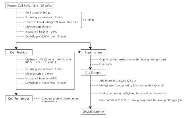
Fig. 1 Sample Preparation Procedure for GC/MS Analysis
