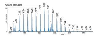
Fig. 2 Alkane mixture (GC-standard, same mass of each component) Asterisks (\*) indicate silver clusters.
