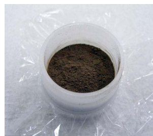
Fig. 3 Seaweed Hand-Pressed (Easy Press) into Cup
