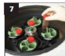
7 Centrifuge at 4000 rpm for 5 minutes
