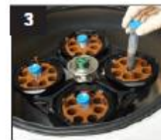
3 Centrifuge at 4000 rpm for 5 minutes
