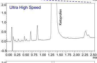
Column : ODS (50 mmL, x 2.1 mm I.D., 1.8 µm) Mobile Phase : 0.1% Formic acid in Water/
