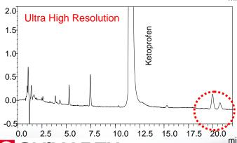
: ODS (250 mmL. x 2.1 mm I.D., 1.8 µm) Column
