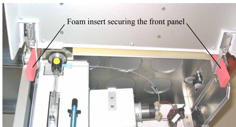
Fig. 2: Foam insert for the front panel (here in a WPS-3000PL)
