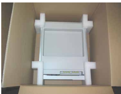
Fig. 27: Solvent rack with foam braces
