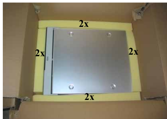
Fig. 23: Autosampler placed and protected in the box
