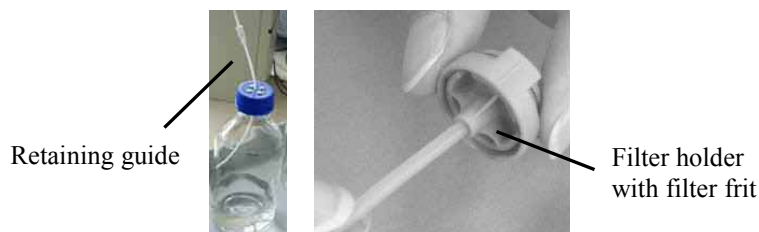
Fig. 3: Connecting the solvent lines to the reservoir
