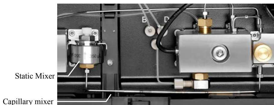
Fig. 5: Two-step mixing system (here in an HPG-3400SD)
