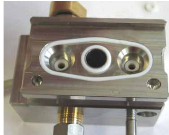
Fig. 48: Seal installed in the pump head
