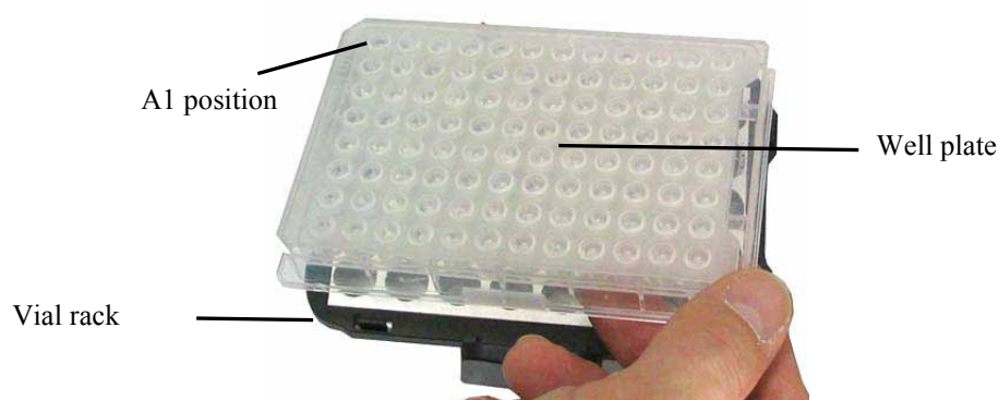
Fig. 19: Installing a well plate on a vial rack
