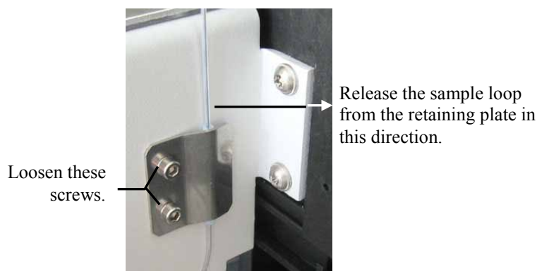
Fig. 55: Sample loop retaining plate
