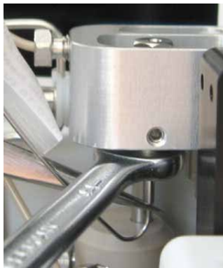
Fig. 76: Tightening the needle seat capillary
