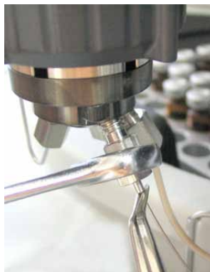
Fig. 78: Connecting the needle seat capillary to the injection valve
