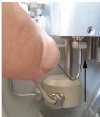
Fig. 73: Inserting the needle seat capillary
