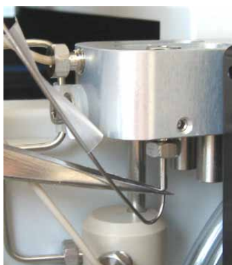
Fig. 75: Aligning the needle seat capillary
