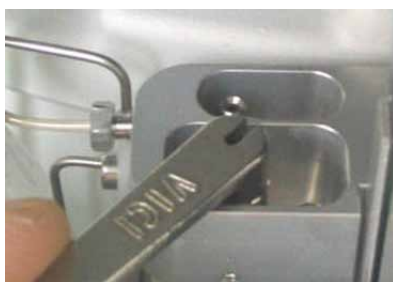
Fig. 63: Removing the retaining screw
