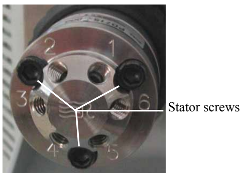
Fig. 85: Stator screws (here on a stainless steel valve)
