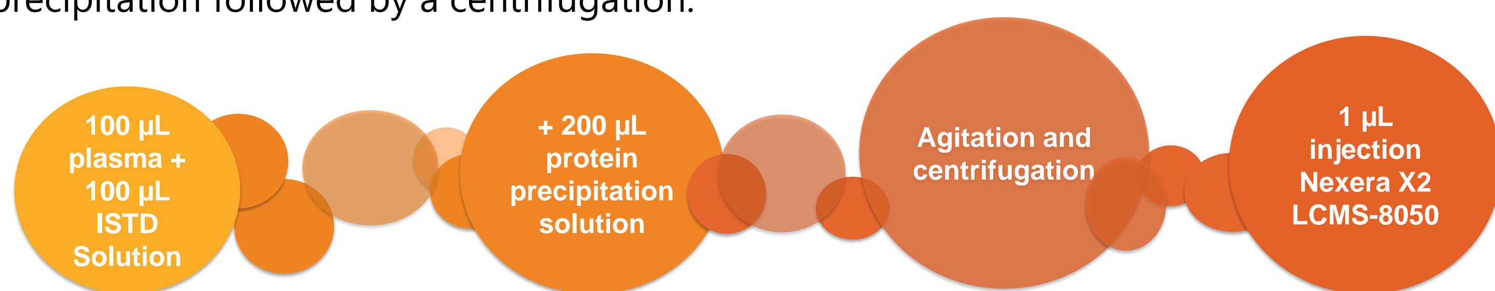
Figure 1. Sample workflow overview for the quantification of amino acids in human plasma.
