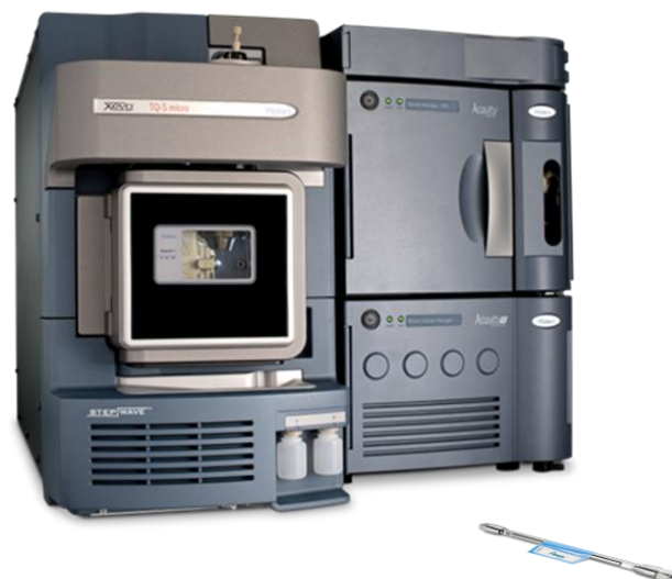
Figure 2: Xevo TQ-S Micro with Acquity UPLC H-Class Plus, Atlantis™ Premier BEH C18 AX 100 mm X 2.1 mm, 2.5 µm column
