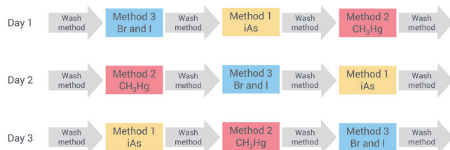
Figure 3. Experimental flowchart for the automated multi-method HPLC-ICP-MS sequences run over three days.
