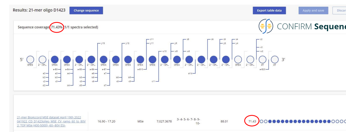
Figure 5. Dot-map sequence coverage (~70%) obtained from high energy MS E untargeted fragmentation. All precursors of the 21-mer heavily modified oligonucleotide (see Figure 2B) were fragmented using an optimized cone voltage ramp (from 60 to 80 V) applied to the Step Wave of a BioAccord TOF instrument.
