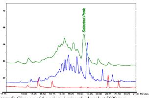
Figure 5: Close-up of the selected mineral oil peak at 5000 ppm
